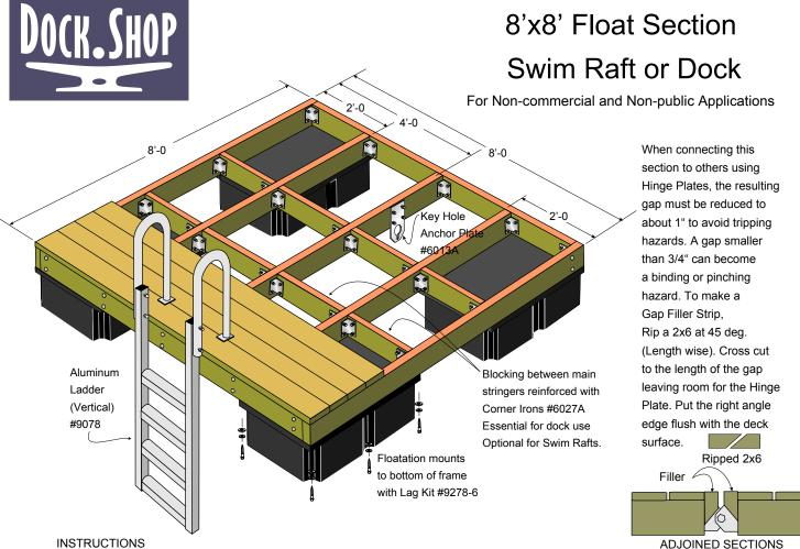
Typical framing to be of grade #1, P.T. min. with 2x6 for non-commercial, light load.
